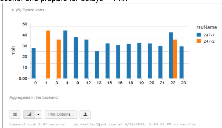
Figure 5. Vehicle Speeds <50 mph observed by roadside units
