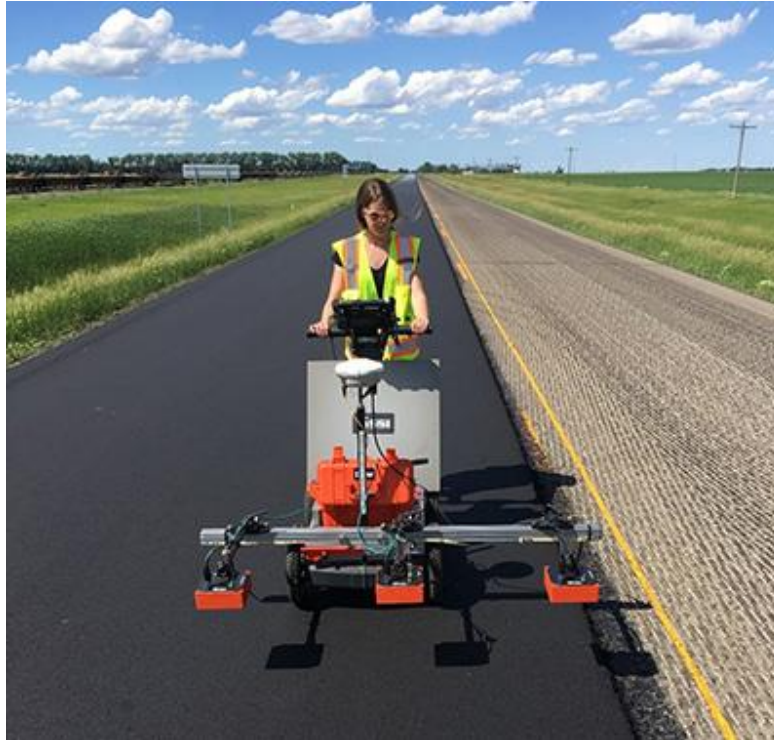
Figure 6: Dielectric Profiling System being used on new pavement (photo credit: Minnesota Department of Transportation)
