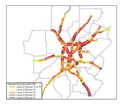
FIGURE 1: "The Challenge"-- General purpose lane level of service, 2030 PM peak hour
