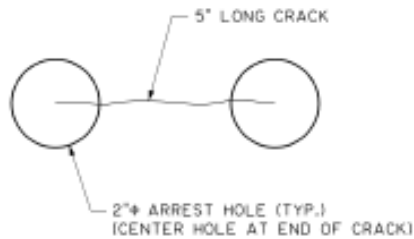
DRILL PATTERN - 5" LONG CRACK
