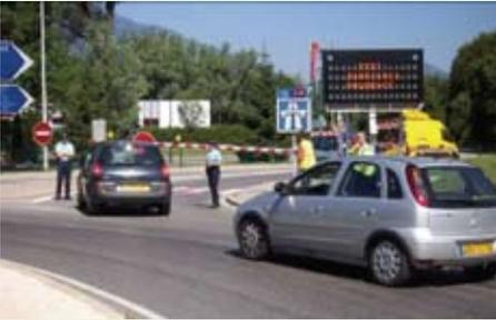
Figure 7: When a ghost driver alert is sent out, motorway operators attempt to confine the problem immediately by activating electronic signs at roadway entry points and closing access to the road using physical barriers.
