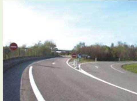
Figure 1: To indicate the correct path to motorists, two “B1” red no-entry signs and a “J5” blue directional marker in the diverging area are positioned side by side. Additionally, directional arrows are painted on the pavement. Both the B1 and J5 signs are well known among French drivers.
