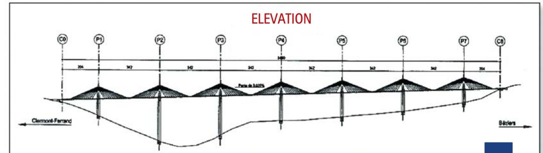
Each reinforced concrete pier stands on a rectangular reinforced concrete footing 3 to 5 meters thick. Each footing has four reinforced concrete foundations, 5 meters in diameter and 10 meters
